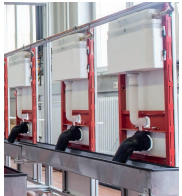
Twelve flushing positions – all with TECE cisterns – have been working in the new flushing laboratory at the Esslingen University of Applied Sciences since mid-2014.
